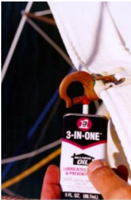
A dab of 3-in-One oil on storm headsail hanks keeps them working freely.
