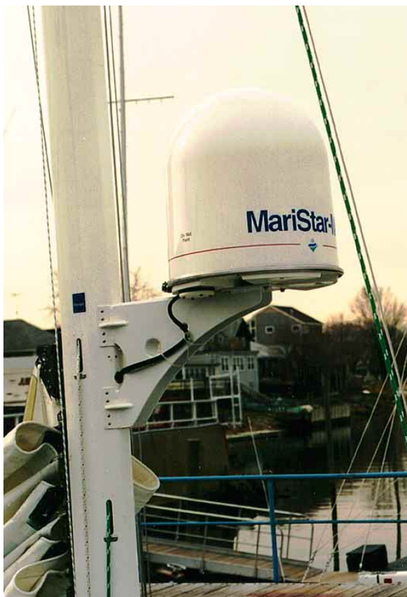
The SatCom M antenna is compact enough to be functional on vessels 50 feet (13.4 m) and larger.
