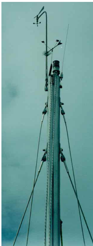
This extension on Beowulf 's masthead instruments made them much more accurate.
