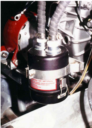
A Racor Crank Vent mounted on a 50-horsepower Yanmar diesel (left). The drawing (right) shows the foam-like media used to precipitate oil out of the crankcase emissions.
