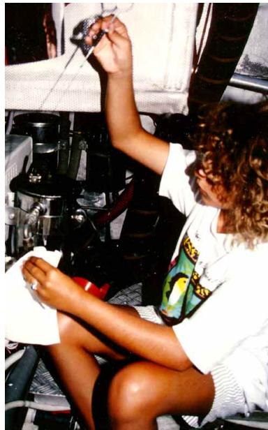
Sarah checking the oil on Sun-deer's Isuzu diesel. We make it a habit to check all liquid levels on the engine before starting the engine each time, and every six hours when powering for long period.
