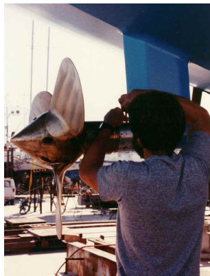
Beowulf's VP2 Hundested (above) and the VP4 on Galatea (below) — highly efficient under power, but approximately 75 percent more drag under sail than a comparable Maxi Prop with streamlined blades.
