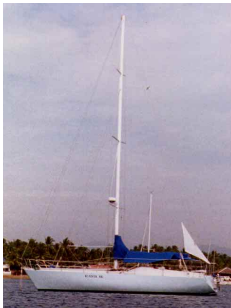
Eos II was of unidirectional glass and foam construction to an Eva Hollman design. Note the “back staysail” being flown from the backstay as a riding sail.
