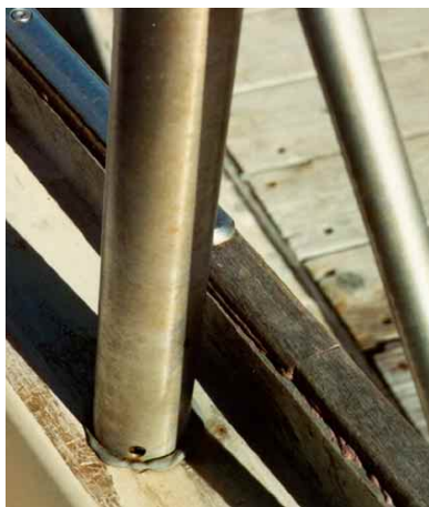
The hull-to-deck joint (on the inside) is fiberglassed over the bolts to make sure it is watertight. The lifeline stanchions are very heavy-duty and do not leak (left photo).
