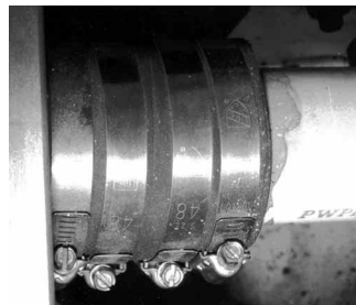
Three different standpipe details. Left: A welded assembly on Sundeer . The 2-inch (50mm) pipe at the top receives all bilge, sump, and galley sink pump discharges. The smaller welded pipe at the bottom is the toilet discharge. There was some question if this would prove a problem, mixing the two types of effluent. However, it never became an issue. The center and right photos show Sundeer 56 and 64 standpipes. These are fiberglass pipes, laminated to the hull skin, with PVC manifolds hose-clamped to the top.
