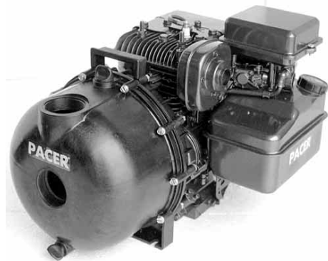
A Pacer gas-driven "de-watering" pump. With a plastic body and impeller, it is ideal for the marine environment. And this unit will pump more than 150 gpm (580 liters/minute).
