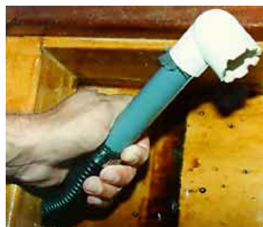
A bit of PVC pipe makes an excellent pump pick-up.
