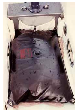
Bladder tanks need a smooth, constrained space. Although high, the cockpit well makes an excellent temporary location.
