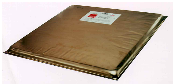
An Owens-Corning Aura insulation panel. This is the most efficient insulation available, with "R" factor of 60 for 1-inch (25mm) thick panels. (Glacier Bay Photo)
