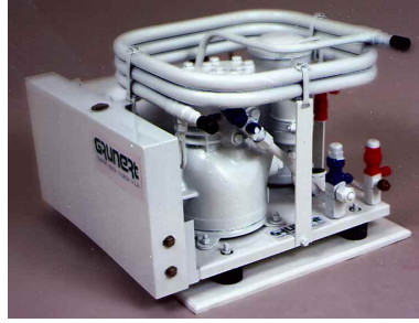
A sealed AC compressor does not have shaft-seal or hose-maintenance problems. However, it is 15 to 25 percent less efficient than a pure DC system. (Marine Air/Grunert photo)
