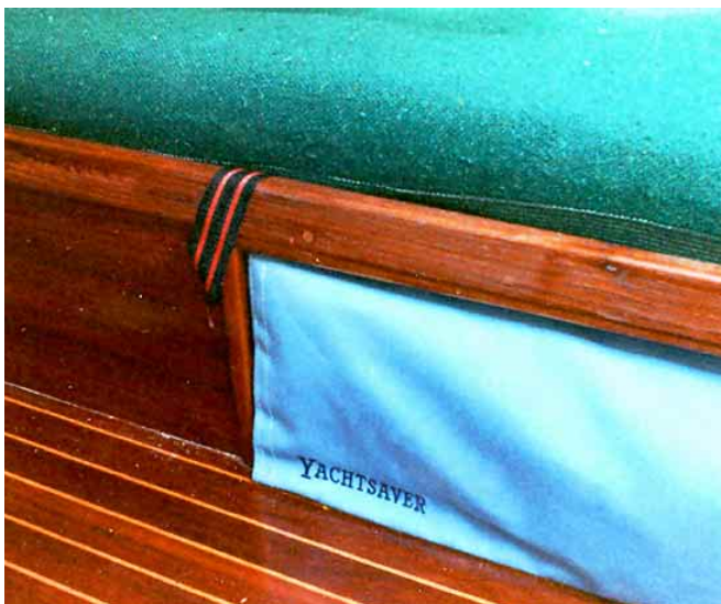
Built-in system installed in recesses of bunk fronts on a J/29. (Yachtsaver photo)
