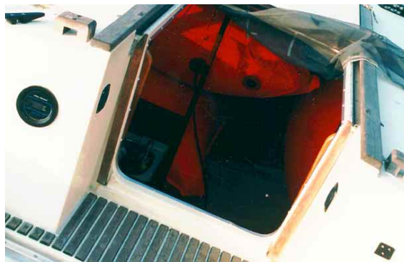
A series of inflatable bags were stuffed into the aft quarterberths and main saloon, and then inflated. (Yachtsaver photos)
