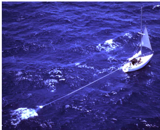
The parachute sea anchor is an effective means of holding station in moderately severe weather. However, most vessels are better running off at speed (assuming they have sea room) in truly severe conditions. (Paratech photo)
