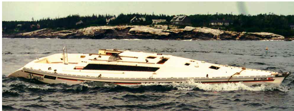
The boat was then towed off on the next tide and brought to a local yard, where she was hauled. Note the bow-down attitude. This is the result of much of the buoyancy in the bags being aft of the hull's center of gravity. (Yachtsaver photo)
