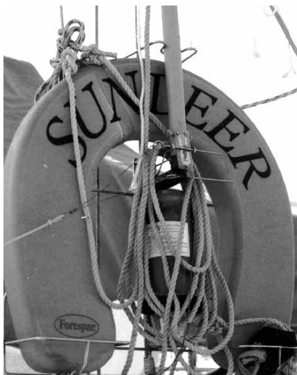
Sundeer's traditional MOB system with a Forespar launcher. A single pull on the lanyard deploys pole, strobe light, horseshoe, and sea anchor. Offshore, we fasten this to the top of our lifelines to keep it clear of any breaking seas. Onshore, we drop it down to deck level.
