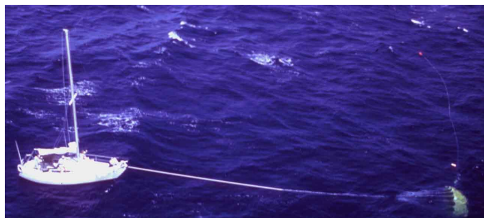
The parachute sea anchor is an effective means of holding station in moderately severe weather. However, most vessels are better running off at speed (assuming they have sea room) in truly severe conditions. (Paratech photo)
