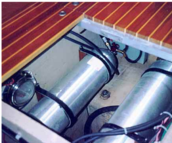
This installation is on an Alden 50. CO 2 tanks are installed beneath floorboards, while the deflated bags are stowed into pockets below the saloon seats. (Yachtsaver photo)
