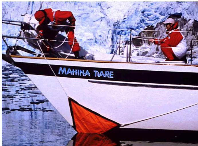
A triangular collision patch being tried out aboard John Neal's Mahina Tiare . Small patches are easier to keep in place against wave action. However, one this small would only work for a very small breach.
