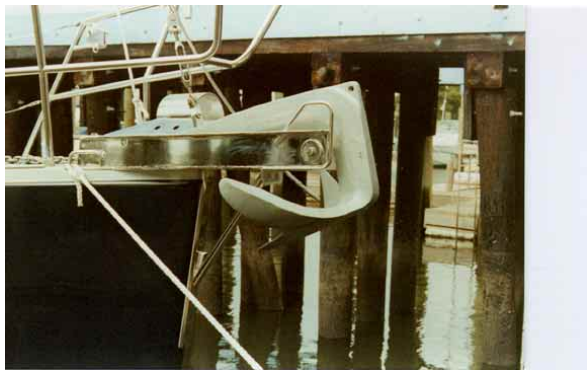
On the Sundeer 64 we worked on a built-in anchor wash-down system. It was never totally successful, as we didn't find the right combination of nozzle design and pump pressure. However, the concept is still valid.
