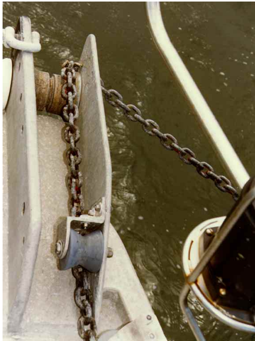
When designing the bow-roller assembly you always have to keep in mind a tide-bound situation, where current and wind fight and you end up with the chain at right angles to the boat. In this case high cheeks or some form of a guard must be built in to keep the chain from jumping off the bow roller and pulling back down the deck.
