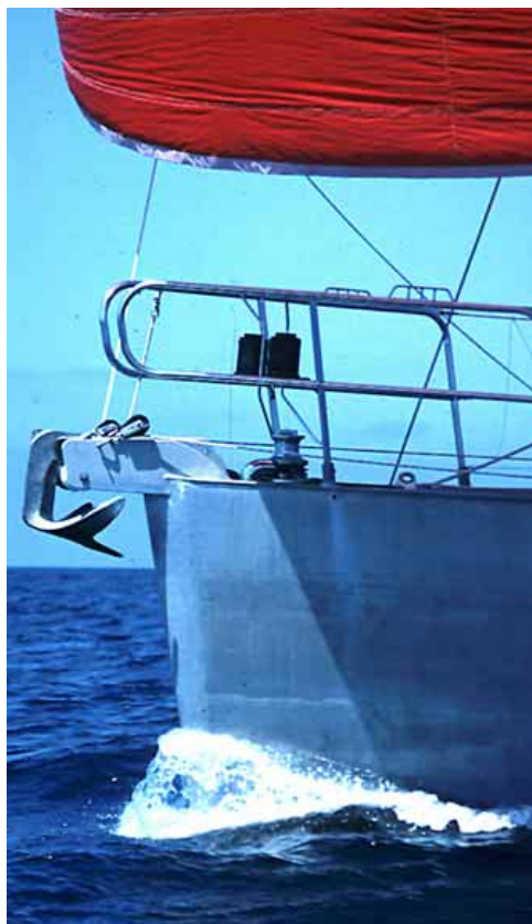
Sundeer's 110-pound (49.9kg) Bruce anchor is well supported by an aluminum weldment made up from 3/4-inch thick (19.1mm) plate. The miniature bowsprit keeps the anchor clear of the vertical stem when the anchor is raised.
