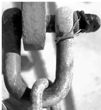
Proper seizing of the anchor shackle with chain and nylon is essential. We like to use flexible stainless wire and then tape over the ends to prevent snagging of light sails.
