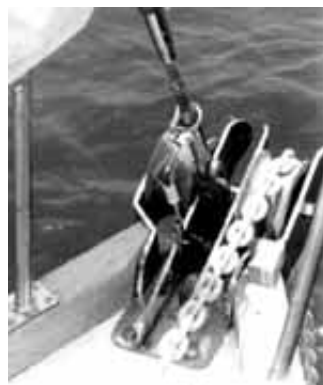
The larger the bow roller, the less friction the chain will see. This 6-inch (152.4mm) roller is ideal for 3/8" (9.6mm) chain.
