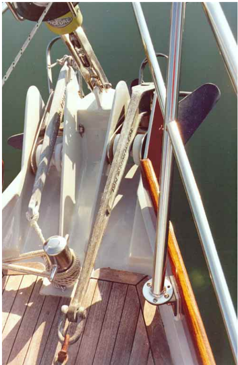
Dual anchors are always difficult to work into a stem-head fitting on a permanent basis. Here two CQRs are ready to go.
