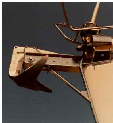
On the Sundeer 64 we worked on a built-in anchor wash-down system. It was never totally successful, as we didn't find the right combination of nozzle design and pump pressure. However, the concept is still valid.
