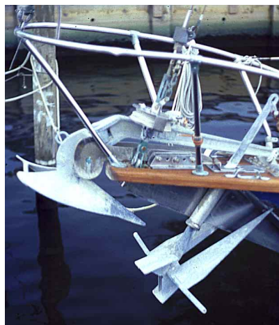
Intermezzo carried both CQR and Danforth anchors on the bow, giving us an easy choice in a variety of conditions. Today we would carry a single bigger anchor.
