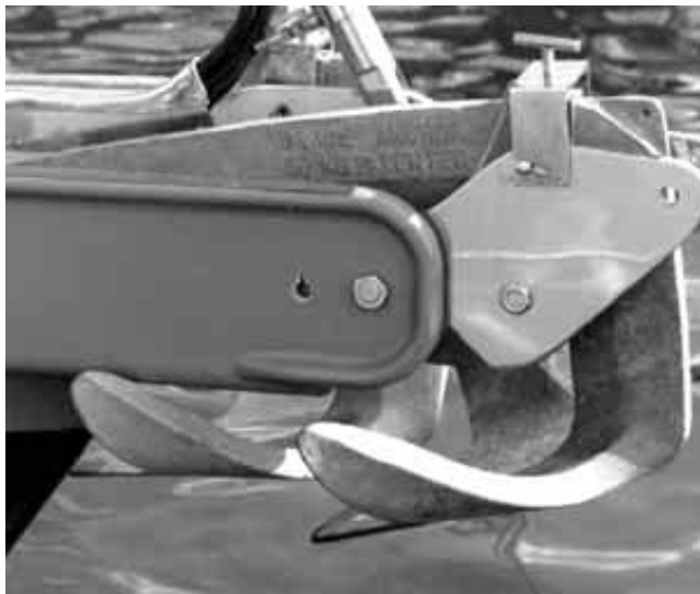
Twin 110-lb. (50kg) Bruce anchors rest side by side on Maya's bow. By staggering the starboard hook slightly forward either anchor can be deployed without interfering with the other.
