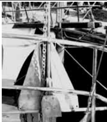
Aboard Intermezzo II we carried the stern anchor mounted on the pushpit. It was easy to deploy and out of the way in this location.
