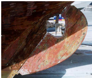
The bottom hinge of a keel-attached rudder is vulnerable in a grounding. When this is loosened or broken, the rudder becomes useless (a not-uncommon occurrence with full-keeled designs).
