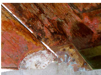
The bottom hinge of a keel-attached rudder is vulnerable in a grounding. When this is loosened or broken, the rudder becomes useless (a not-uncommon occurrence with full-keeled designs).
