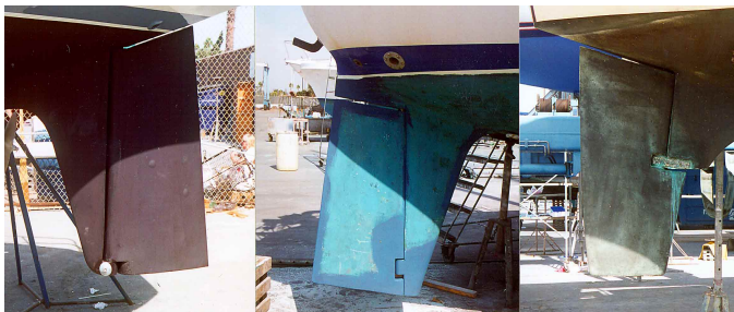
Three types of skeg-mounted rudders. The left photo shows a bottom detail which will quickly fail in a grounding, leaving the boat without steering. If the rudder swings back and forth on the upper bearing, a hole is likely to be torn in the hull bottom, which could lead to a sinking if not quickly dealt with. The middle design is marginally safer. The right photo shows the correct detail with the bottom rudder hinge midway up the rudder. Also, the projection forward of the rudder shaft on this design will contribute counterbalance and reduce steering forces.
