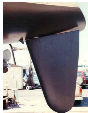
Sundeers spade rudder, a massive aluminum weldment, is capable of taking more grounding loads than just about any normal skeg.
