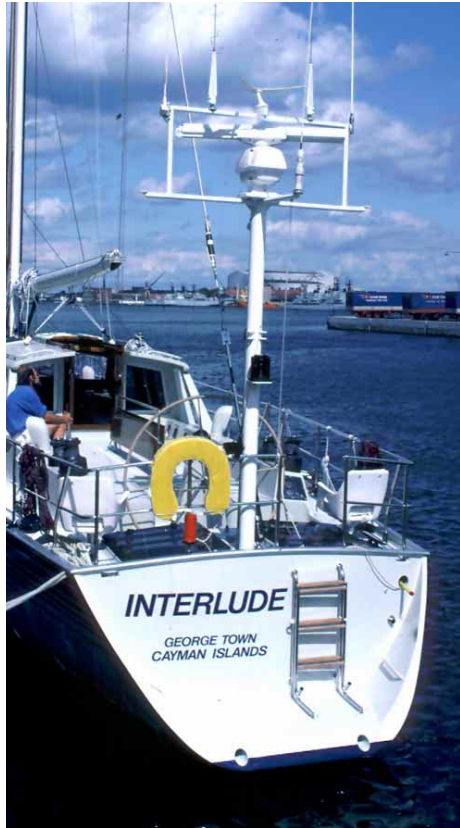
One of our early Deerfoot 74 designs with a very short stern overhang. This is a faster shape in light airs under sail than a transom which touches as there is less wetted surface. But it is slower under power and at speed under sail because the effective waterline is shorter. It also forces you to a less favorable distribution of buoyancy throughout the hull shape.
