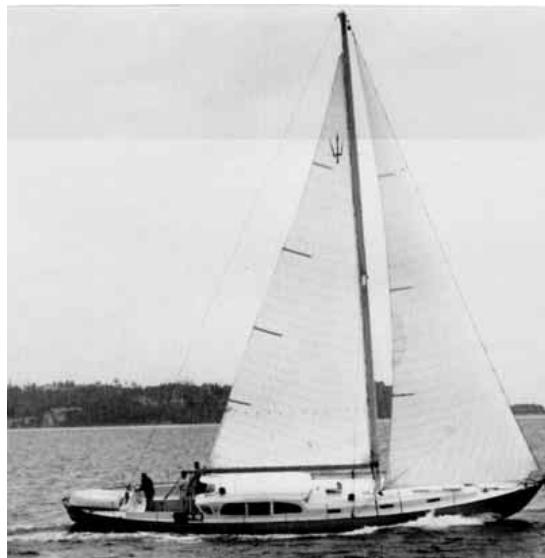
Bill Garden's Oceanus was a design that was ahead of her time. She was 60 feet (18.5 m) overall, with a 12-foot (3.7m) beam, a 48-foot (14.8m) waterline, and a draft of just 6 3/4 feet (2m). She displaced 36,000 pounds (16,326 kg) and had a displacement-length ratio of 145.
