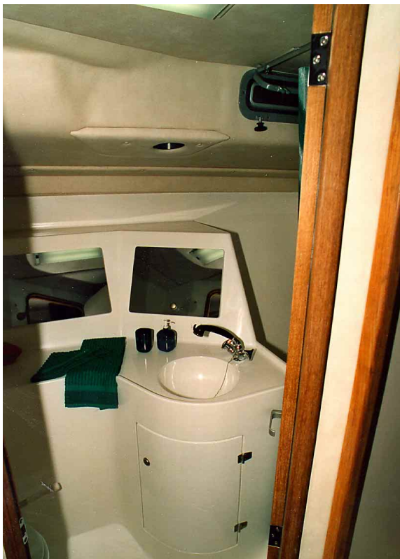
The aft head is quite large. There's a toilet at the forward end (well wedged in for use at sea). The sink and vanity provide plenty of space for doing all those things that are required before going out on the town. At the aft end of the compartment is a shower area with room for a compact washer/dryer.
