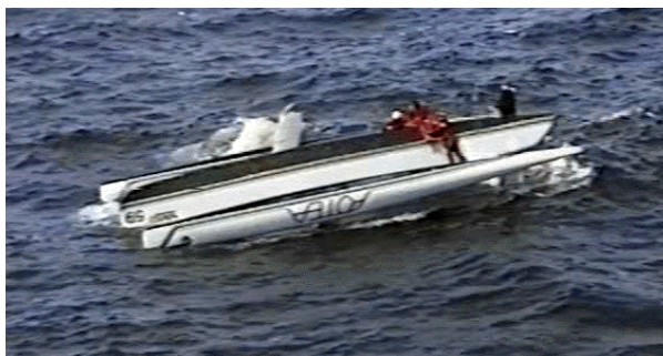
Beowulf VI was a big step up from the open trampoline boats we sailed before. She was 39 feet (12 m) long and weighed just 2,140 pounds (970 kg) all up in cruising trim! She had a displacement-length ratio of 20 and could carry 10 square feet of sail for every square foot of wetted surface!
