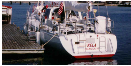
A Sundeer 64 (above) at rest in Newport, Rhode Island. She's at about 90% load here ready to head for the Virgin Islands. About three inches (75 mm) of the transom is immersed in this trim.
