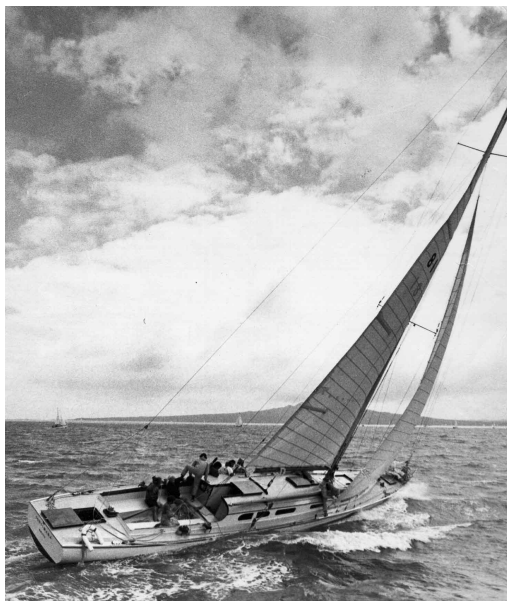
Innismara driving to weather in a fresh breeze. She has a beautifully clean wake, no stern wave to speak of, and a very small bow wave. Look at how little fuss her hull makes going through this afternoon chop. She is sailing with a full main and staysail, in effect an extreme fractional rig (although she had a masthead headstay for light airs). This is a rig configuration that the French "invented" 30 years later for their BOC boats. (Sobstad New Zealand photo)
