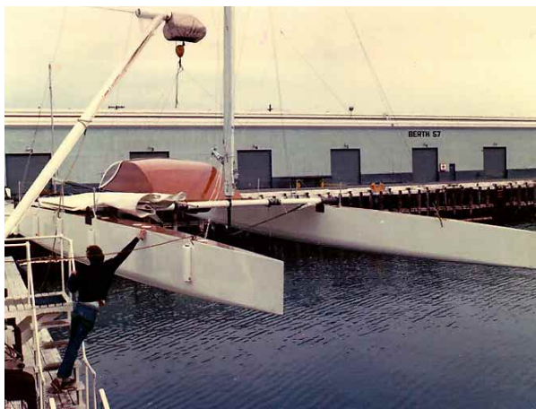
Beowulf VI was a big step up from the open trampoline boats we sailed before. She was 39 feet (12 m) long and weighed just 2,140 pounds (970 kg) all up in cruising trim! She had a displacement-length ratio of 20 and could carry 10 square feet of sail for every square foot of wetted surface!
