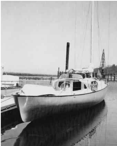
Bill Garden's Oceanus was a design that was ahead of her time. She was 60 feet (18.5 m) overall, with a 12-foot (3.7m) beam, a 48-foot (14.8m) waterline, and a draft of just 6 3/4 feet (2m). She displaced 36,000 pounds (16,326 kg) and had a displacement-length ratio of 145.
