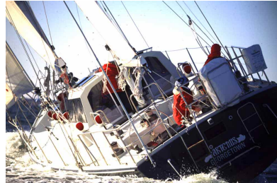
Two views of loaded Sundeer 64s. Above, the boat is close-reaching at about 11 knots, a speed-length ratio of 1.37. The stern wave is starting to stretch out behind the boat and is quite small in magnitude.
