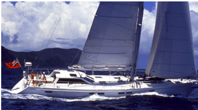
Evolution , a Chuck Paine–designed 66-footer (20.3 m), is reaching in 20 knots of beam wind. She’s carrying a blade jib with reefed main and doing about 10 knots in this photo. (Chuck Paine photo)
