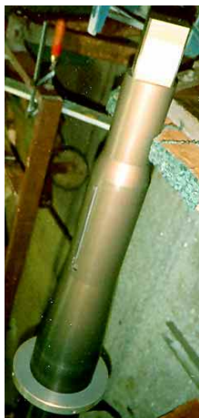
Top two photos: This rudder shaft and matching collar will later be welded into the hull. The slot in the rudder shaft is at the bottom and will accept flat-plate extension of the shaft, forming a structural spar to which the ribs and plating of the rudder are eventually welded.
