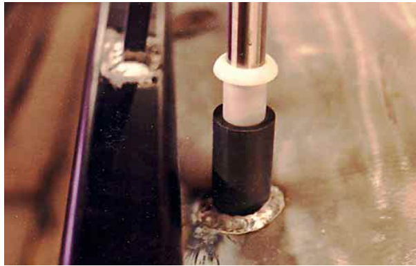
Two views of a lifeline-stanchion socket (above and left) — welded to the deck and to a frame below the deck. A nylon insert isolates the stainless stanchion from the aluminum socket.
