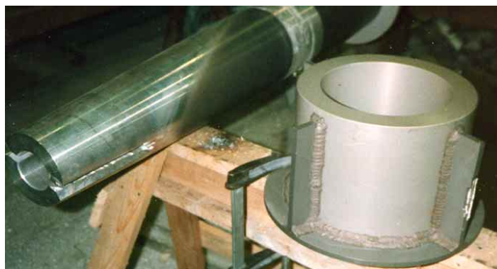
Top two photos: This rudder shaft and matching collar will later be welded into the hull. The slot in the rudder shaft is at the bottom and will accept flat-plate extension of the shaft, forming a structural spar to which the ribs and plating of the rudder are eventually welded.
