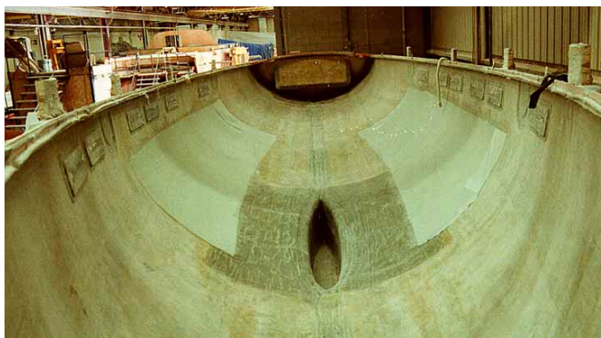
The hull of a Sundeer 64 after molding has been completed. You can see the solid area of laminate around the keel. The long rectangular patches in the turn of the bilge are where the water tanks will be bonded in.
