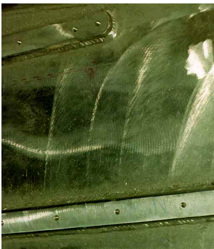
These jib-track bases (left) are 3/8-inch (9.6mm) plate that have been drilled and tapped to match the mounting holes in the jib track. These plates have been welded to the top of the deck in order to prevent leakage between the fasteners and the interior.
