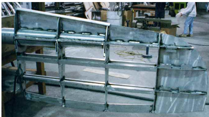
Top two photos: This rudder shaft and matching collar will later be welded into the hull. The slot in the rudder shaft is at the bottom and will accept flat-plate extension of the shaft, forming a structural spar to which the ribs and plating of the rudder are eventually welded.
