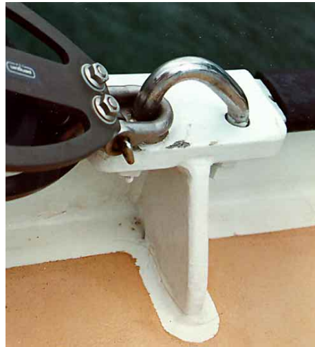
An interesting detail for attachment of turning block to the deck (above). Note the shape of the U-bolt. The aft leg is angled to help restrain the entire structure against forward pull.
