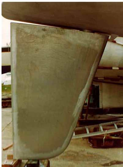
You may want the rudder to have its own zinc. If this is the case, it should be let into a recess, as shown here (above), so that it is flush with the surface. We've built rudders with and without.
