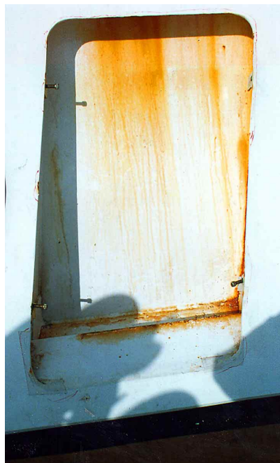
The hull surrounding this doorway has been properly prepared. However, the doorway itself, where the rust is showing through, was not sandblasted before application of the undercoat. (Doug Templeton photo)
