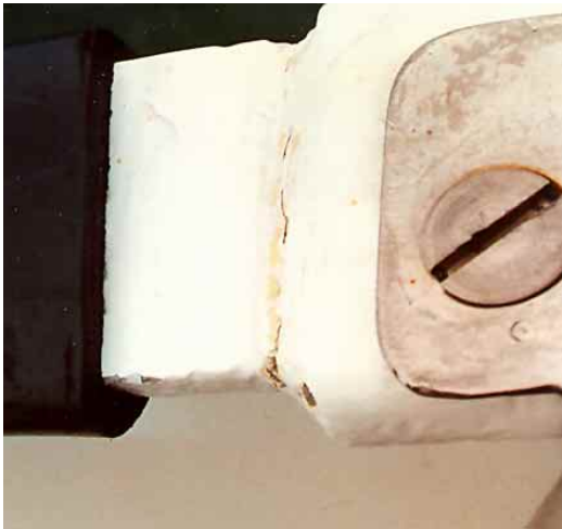
The aluminum toerail (above) is welded onto a high toerail. It projects beyond the topsides a little and has a hard rubber extrusion placed over the edge to protect it and neighbors from the aluminum.
