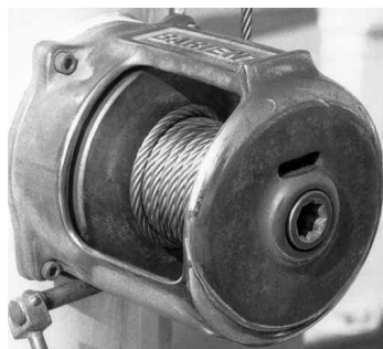
Vintage reel wire winches like this Barient from the '60s are extremely dangerous. They should be replaced at the first opportunity.
