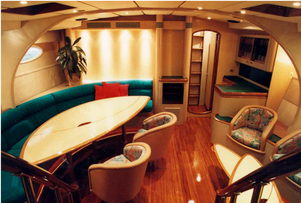
Lighting on this 93-foot (28.6m) cruiser (on which the Harrills did the interior design work) was a big part of the evening ambiance equation. She has hull side lights, an array of dimmer-controlled halogens in the headliner panels, and additional spots designed to wash the bulkheads in light. The light that hits the vertical surfaces is reflected elsewhere, creating a nice atmosphere for very few watts.
