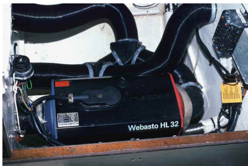
A Webasto hot-air heater. These units work well on yachts up to around 50 feet (15.4 m) in temperate climates and are quite easy to install. The main negative is that the hot-air ducts take quite a bit of storage room.
