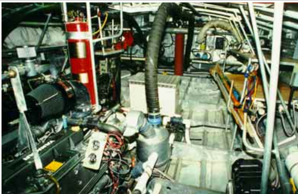
Above: Engine rooms are difficult to photograph, and this one is no exception. This shot is taken from the engine room door, at the back end of the aft port head. The main engine is to the left of the photo. The genset (not seen) sits aft and to the left.
