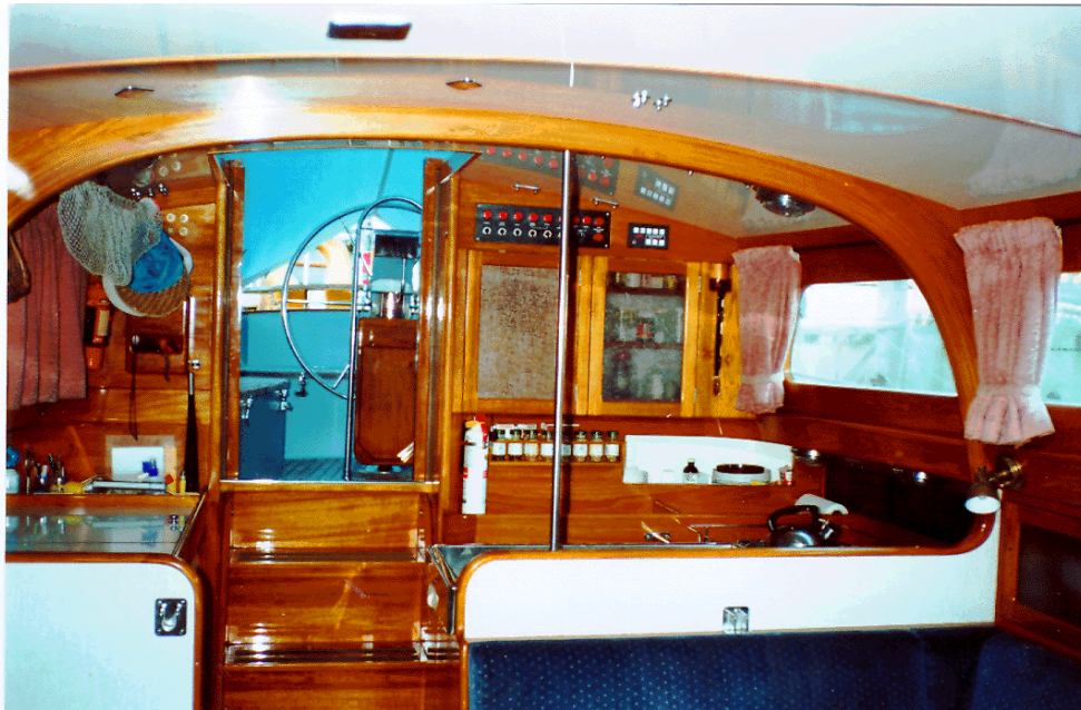
Looking aft (top photo) toward the galley area. The fridge/freezer bow on the starboard side also works as a chart table. The galley layout (lower photo) features a stainless sink and counter, with integral stainless fiddle rails. Easy to clean and you never have to worry about leaks in the caulking
