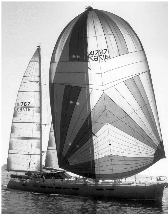
Sundeer's spinnaker was substantial in size, almost 2,450 square feet (232 square meters). We'd carry it in light airs reaching, and in medium airs on a run. One of the keys to handling this large sail was the ATN Snuffer. If the breeze was up, we'd run off square, trim the leech tight against the main to collapse the spinnaker, then ease the pole and guy. With the sail lying docilely against the leeward side of the main, we could snuff the sail without a problem.
