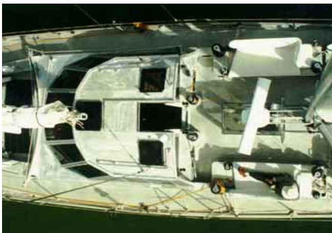
Above: The cockpit area is contiguous with the pilothouse. Sail controls are clustered around the aft end of the pilothouse, where they can be easily adjusted. The large winches at the aft end of the cockpit are for the staysail and main runners. The smaller aft winches handle the mizzen vang.
