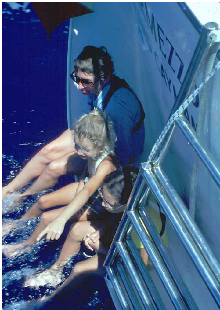
The swim step on Intermezzo II was originally conceived as a way to aid a man-overboard recovery. It was just 20 inches (508mm) deep. We quickly learned how valuable they were for swimming, getting into and out of dinks, and just dragging your feet at sea. Today we typically make these about 50 percent wider.
