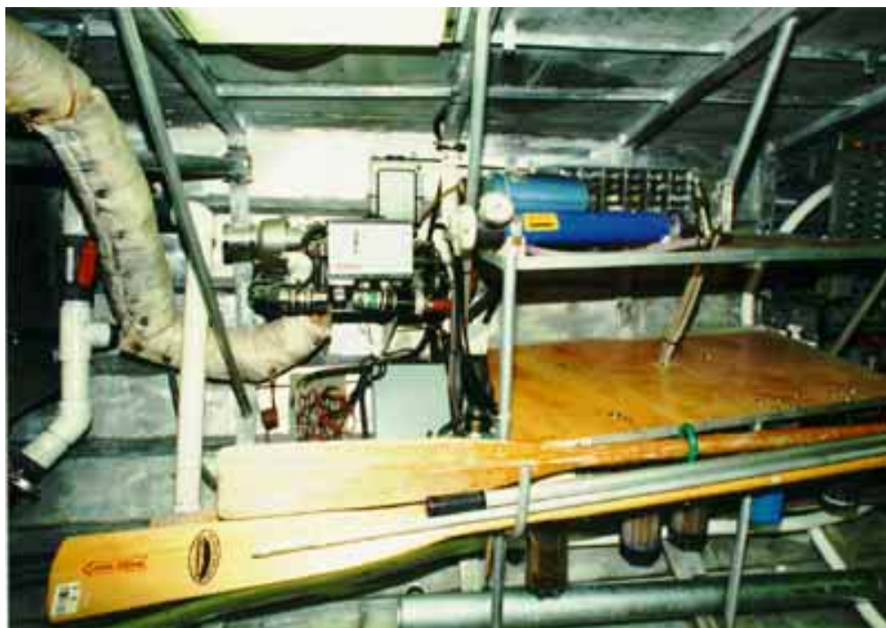
Shelves run along both sides of the hull, on which we stow everything from dive gear to covers. The Teledyne diesel boiler is shown to the left (aft), along with the Village Marine Little Wonder watermaker on the top shelf. A larger 50 GPH (238 liter) unit is mounted below the shelves.
