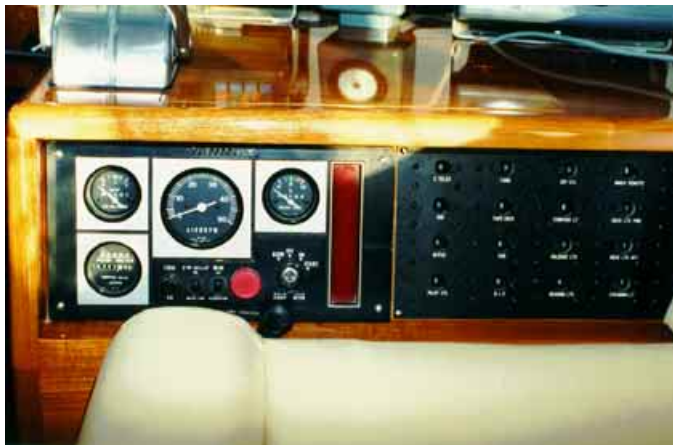
Left: On the starboard side we have the engine panel. Here also are the circuit breakers to control gear that is normally switched when on watch (such as deck lights and electronics).
