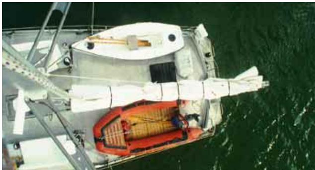
Above: One of the bonuses of this deck layout is proper dinghy storage. We've got space for our hard dink and the inflatable, both of which are launched with the mizzen spinnaker halyards.
