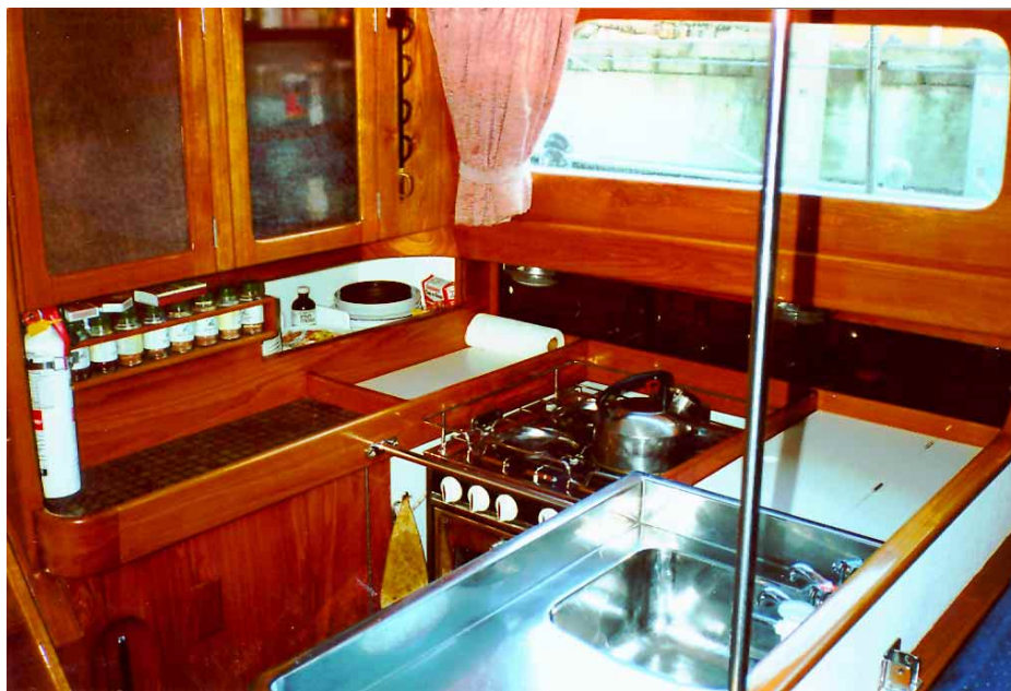
Looking aft (top photo) toward the galley area. The fridge/freezer bow on the starboard side also works as a chart table. The galley layout (lower photo) features a stainless sink and counter, with integral stainless fiddle rails. Easy to clean and you never have to worry about leaks in the caulking
