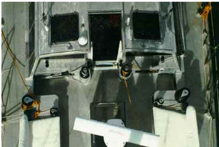
Left: The two winches beside the companionway entrance control the main and mizzen sheets. Both can be trimmed or eased from inside the pilothouse. The larger outboard winches are the primaries, for headsail sheeting and warping when coming into difficult docking situations.
