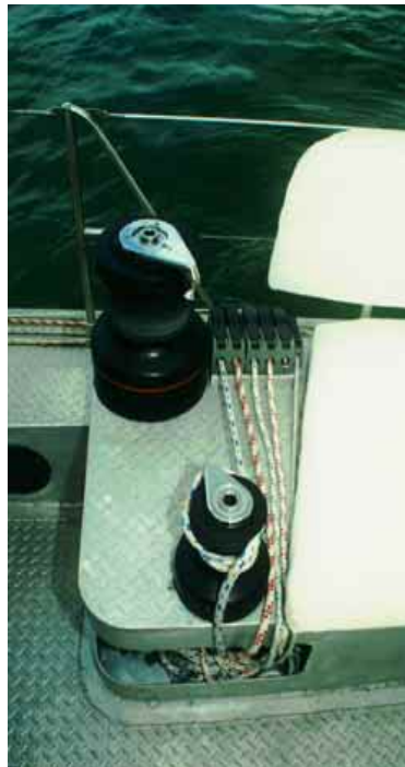
Above: The smaller inboard winch handles a variety of tasks. Inboard and outboard jib sheet adjustment, main sail vang, bowsprit angle, and main runner retriever all end up in this area. Note the rope tail storage under the coamings.
