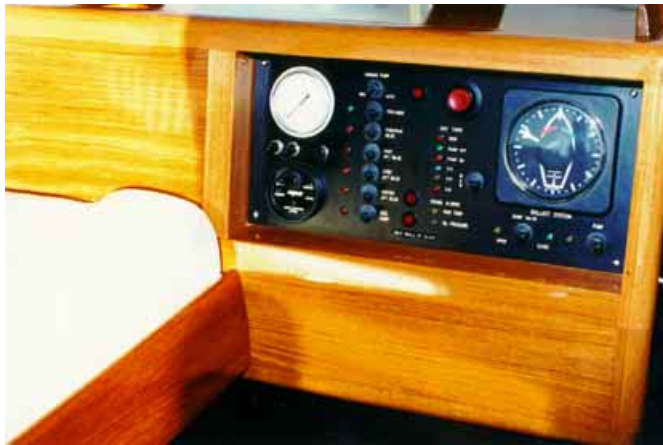
Above: A control panel is let into the face of the port nav cabinet for keeping track of various functions (alarm and otherwise) when on watch. From here we can monitor the bilge pumps, ballast pumping system, fuel day tank signals, etc.
