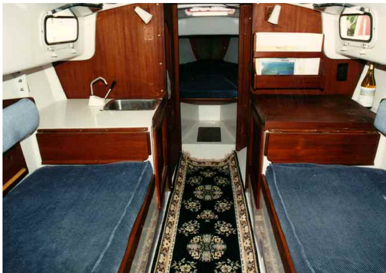
The main cabin of the Contessa 26 is tight, but still offers the comforts of home. There's a nice little sink and galley area to port and a small chart table to starboard. Forward you'll find V-berths and an enclosed head.
