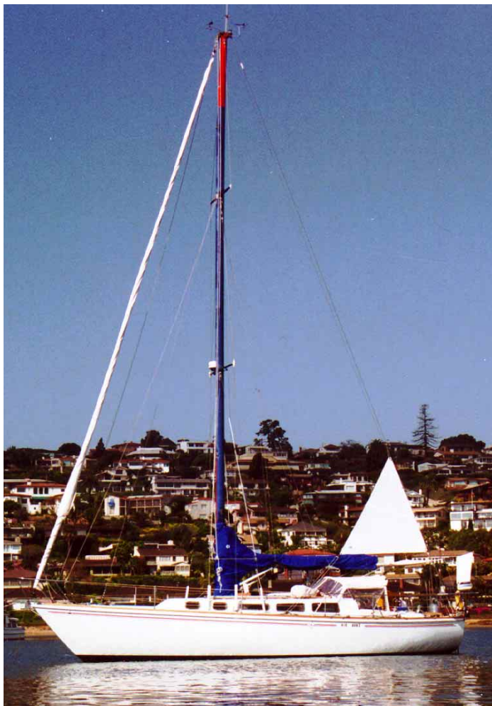
HioAvae anchored in San Diego just prior to heading off for Mexico. The masthead is red for better visibility. Note the riding sail on the back stay.
