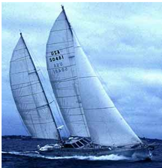
Beowulf at speed, during sea trials, after her interior fit out was completed. She is reaching at 13.5 knots in 18 knots of true wind.
