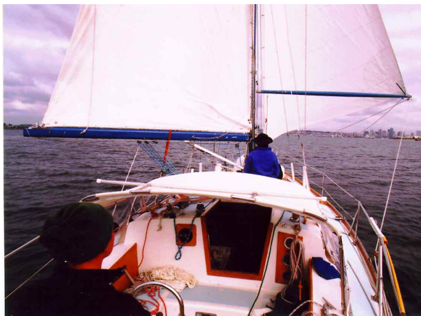
The running rig, 125-percent jib poled out to weather, and the lightweight (3-ounce) genoa staysail sheeted through the end of the main boom. In 10 knots of true wind, the genoa staysail will add 10 to 12 miles to the day's run.
