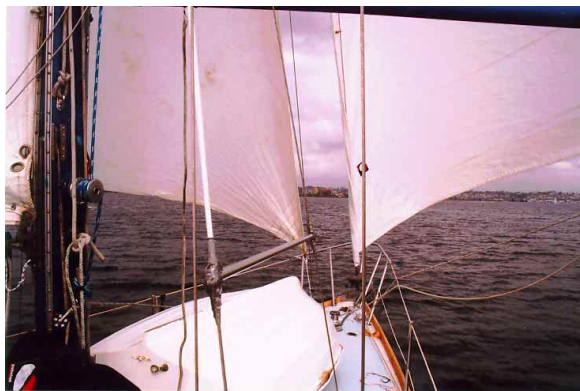
The running rig, 125-percent jib poled out to weather, and the lightweight (3-ounce) genoa staysail sheeted through the end of the main boom. In 10 knots of true wind, the genoa staysail will add 10 to 12 miles to the day's run.
