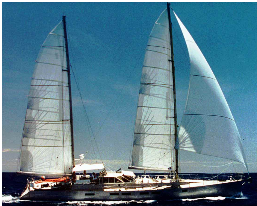
Beowulf is sailing here, en route between the Yasawa Islands and Nandi in the Fiji group, at 10.5 knots with the wind on the quarter. Note the sailing awning covering the cockpit area, and the Novaran inflatable, with 30-horsepower outboard on the aft deck. Our hard dink is to starboard.
