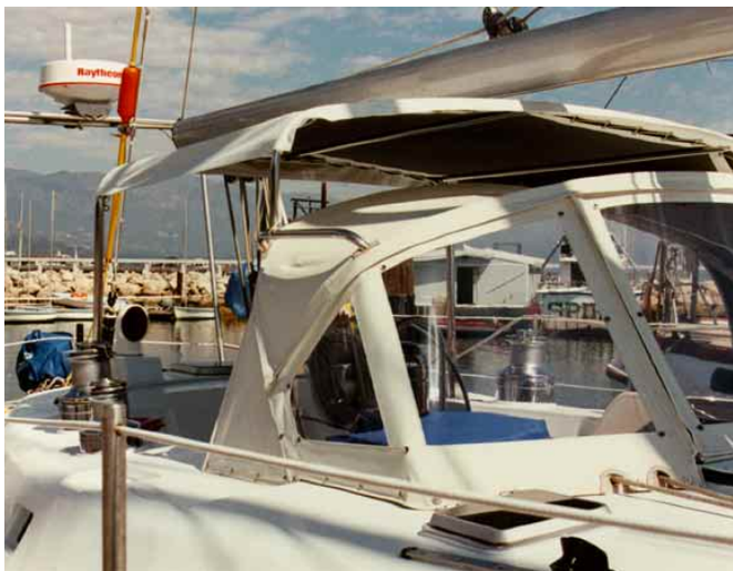
A clever dodger extension here with a frame attached to the dodger aft bow for forward support. The aft end of the awning has its own permanent bow for support.
