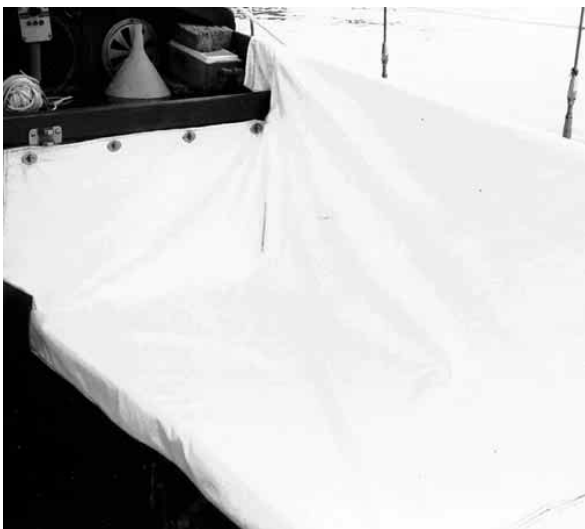
Sue Moesly made these vinyl cockpit-locker covers to keep water from finding its way below during their circumnavigation on the 38-foot (11.7m) Svea.
