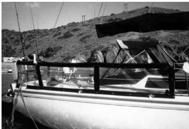
Using dodger window material for weather cloths opens up the cockpit area.
