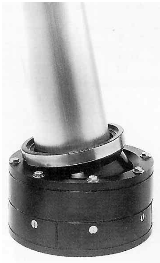
Self-aligning bearings allow for misalignment between the top and bottom bearing, as well as for deflection of the rudder shaft under load.
