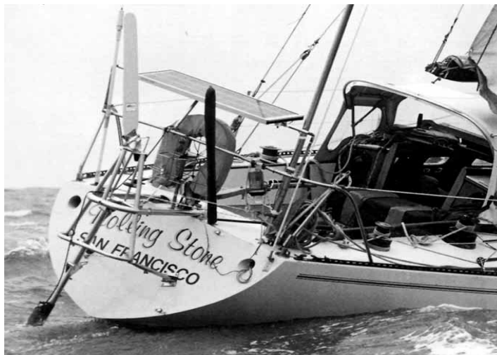
The Monitor windvane is a modern, all-stainless-steel version of Nick Franklin's Aries windvane. The servo pendulum action creates a tremendous amount of power. (Scanmar photo)
