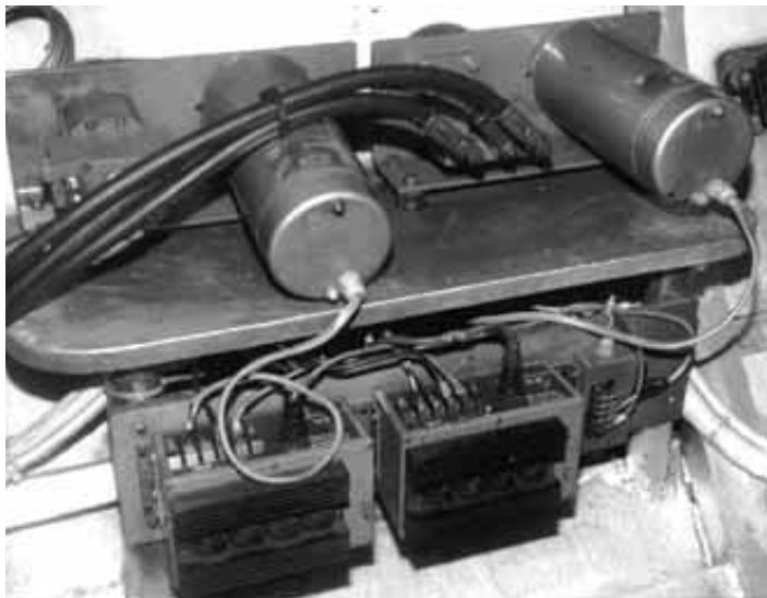
These are twin 1/2-horsepower WH Pilots hydraulic-drive units. Mounted below are the motor controllers. Each of these pumps drives its own ram, giving a totally redundant system.
