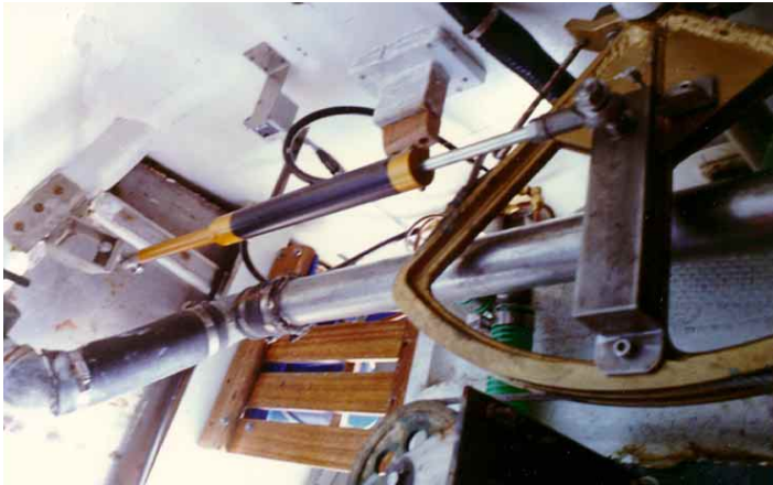
Connecting a hydraulic ram to a conventional quadrant can be accomplished quite easily, as shown here. However, make sure that the spacer bar and its connecting bolts are robust!
