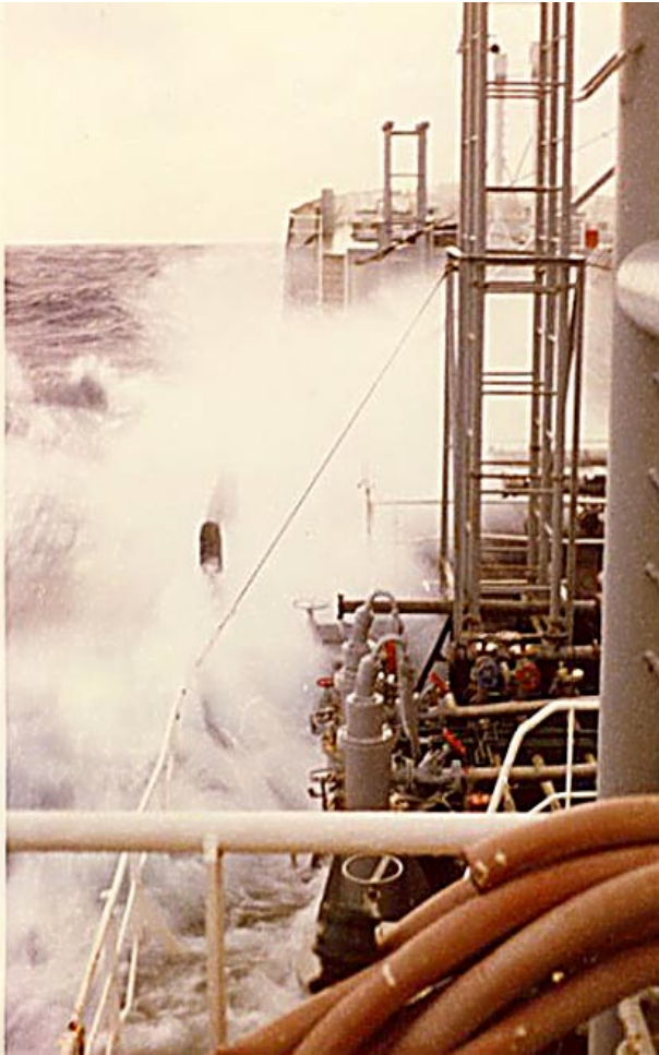
Heavy going in a 5,000-ton chemical carrier. In Hurricane Allen she took water down her 90-foot (27.6m) exhaust stack.
