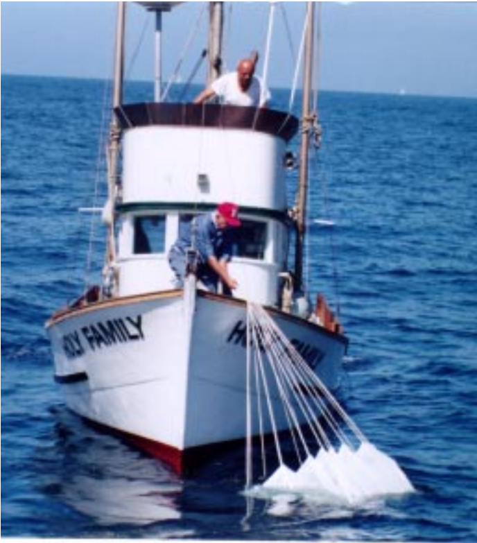
Commercial fishing boats were the first to use parachute anchors for heaving to when drifting at night or when waiting out bad weather.
