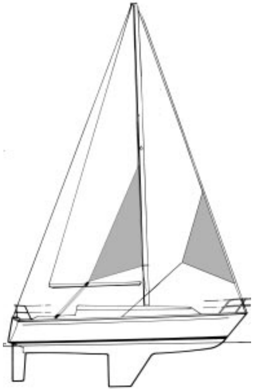
The proportions shown here are for storm-force-and-above wind strength. These sails are smaller in scale than the norm based on ORC regulations.
