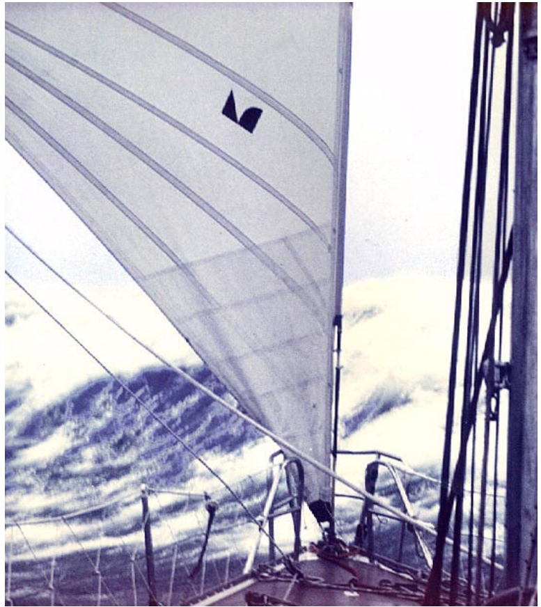
A high-clew storm jib in the furious fifties aboard Ceramco New Zealand in the Whitbread Race. The clew is cut high so the sail will trim well off the wind as well as to windward. A high clew also keeps water out of the foot of the sail.
