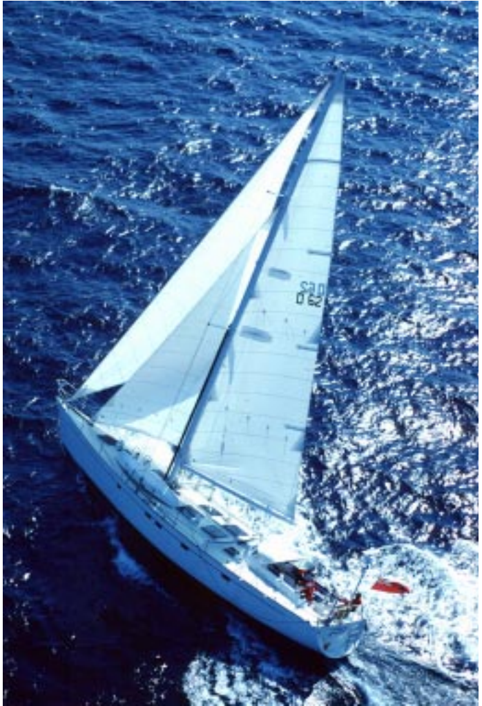
Intermezzo II at speed with jib top, staysail, and full main. This 62-foot (19m) design was considered radical when she first debuted, but in reality was extremely conservative. The primary focus of her design was dealing with heavy weather.
